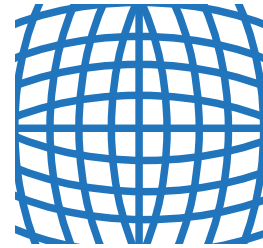
Barrel distortion Negative radial displacement
